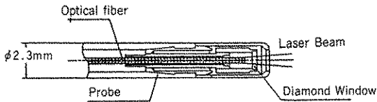
Fig. 13 Cross-sectional View showing Optical Probe.
