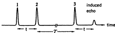
Fig. 3 (a) PHB Molecule as a three-level system. (b) Line shape of molecular spectrum g(\omega) . (c) Configuration of 2-pulse and 3-pulse photon echo observation.
